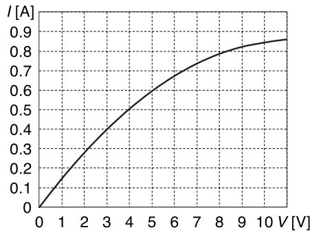
Fig. 5 Example of the characteristic of the current I when the voltage V is applied to the resistance.
